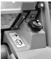
Windscreen washer tank and filler cap + decal.
